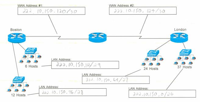
Draw the necessary lines and color in the used squares with different shades to highlight each sub-subnet.
