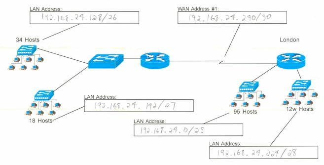
Draw the necessary lines and color in the used squares with different shades to highlight each sub-subnet.
