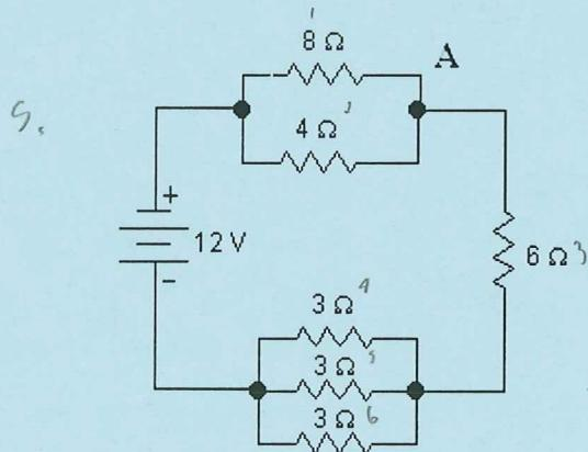
Find the total resistance and total current for each of the above circuits and the voltage at point A.
