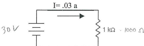
4. Find the total resistance, the current in the circuit and the voltage drop across each resistor.
